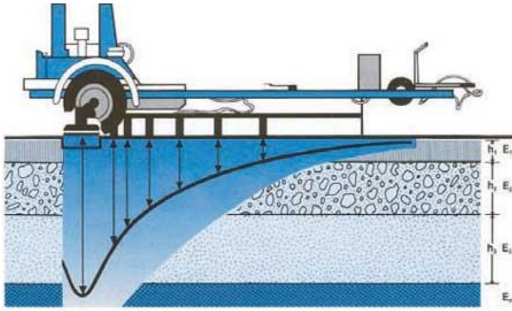
Figure 2. 4: Schematic of a standard FWD test (Dynatest 2016)
